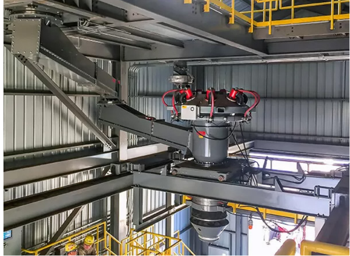
An articulating arm positioner integrated with a DCL loading spout designed for loading multiple vehicle hatches without requiring repositioning of the truck or railcar.
