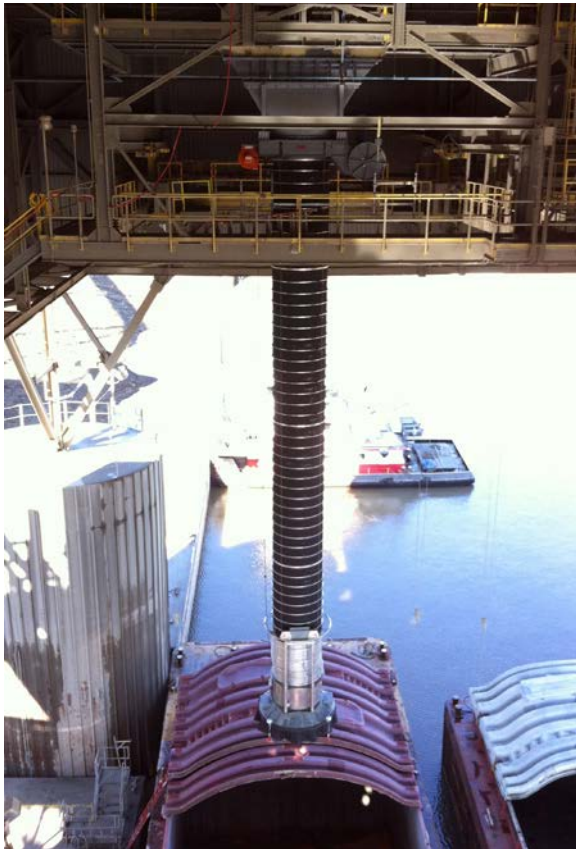
A barge loading system transfers aerated cement at a high loading rate for efficient bulk handling.
