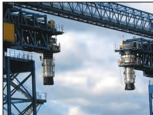
OV style heavy duty loading spouts with compact filter modules on swinging boom.
