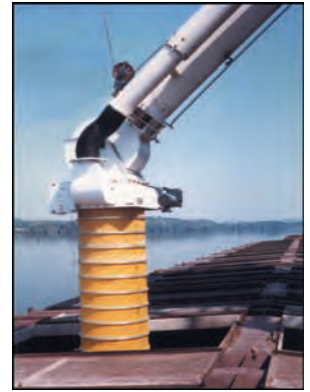
Pivoting gimbal allows different loading angles.
